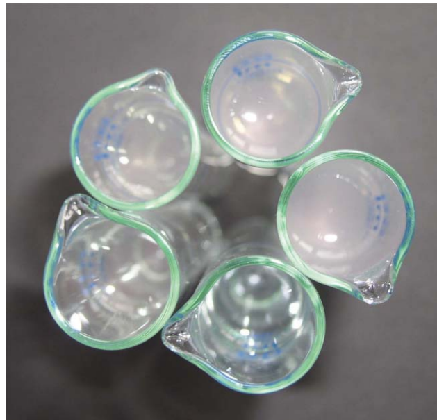
Fig. 5 Colorimetric Nessler cylinders containing standard solutions of NaCl (0, 10, 20, 40 and 60 ppm) for semi-quantitative determination of halides.
