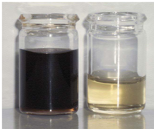
Fig. 1 [C 6 dmim][BF 4 ], before (left) and after (right) treatment with activated charcoal in acetone at room-temperature.
